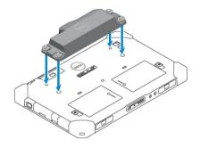
2. Lift up the screw handles and tighten all four screws.
